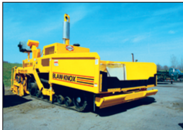
Bituminous Roadways owns seven Blaw-Knox pavers, including this 5510 rubber- track paver, the most recent addition to the company's paver fleet.
