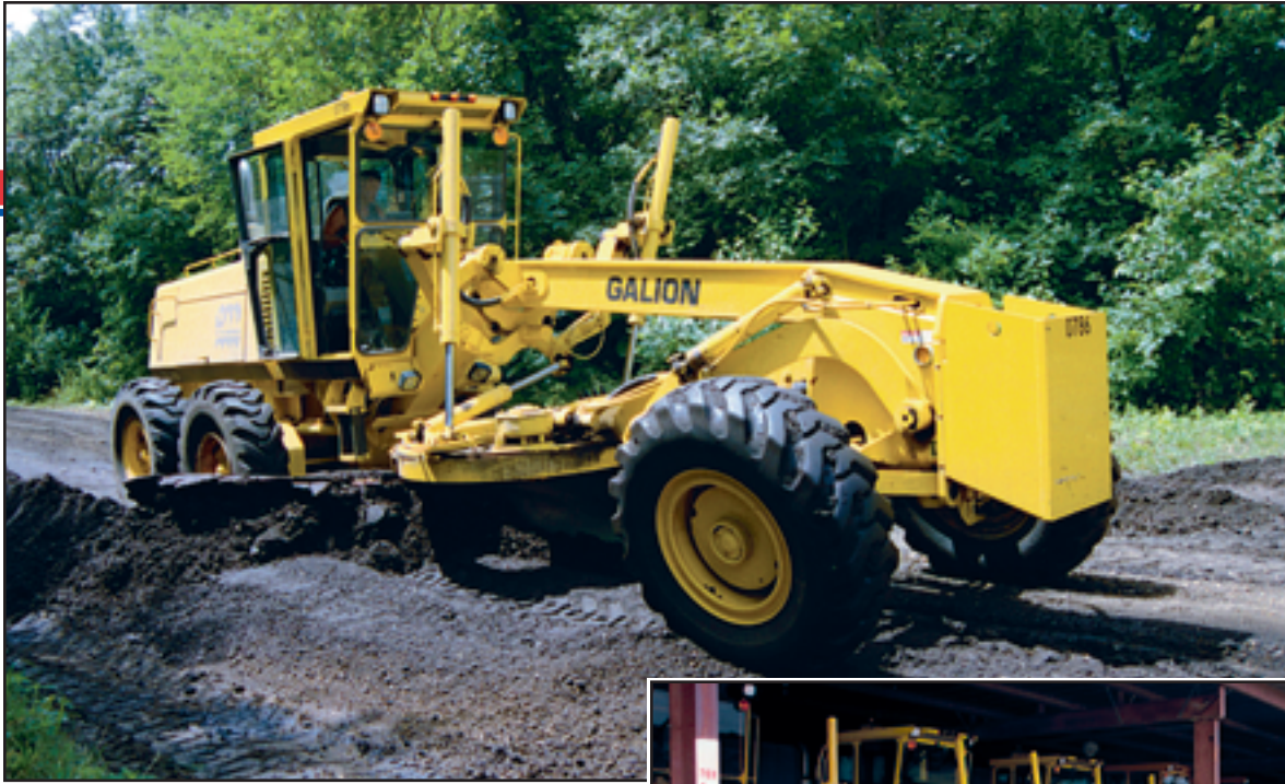
The operator of a Galion 850 motor grader grades a new road on East 38th Street in Des Moines.
