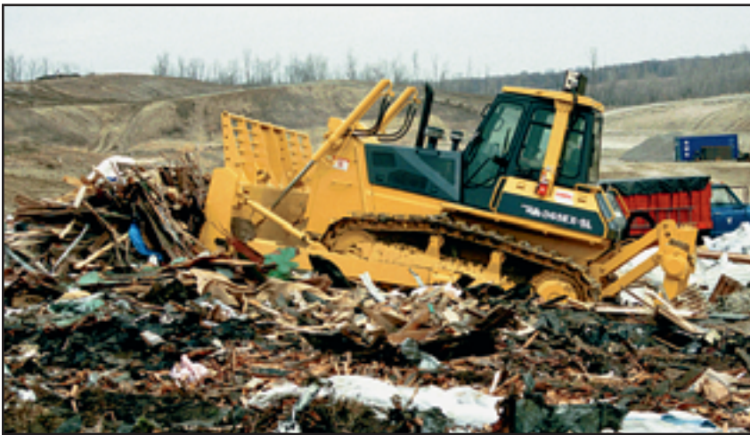
The Komatsu D65 “landfill dozer” is specially outfitted with extra guarding, bracing and plating to withstand the demands of a landfill application.
