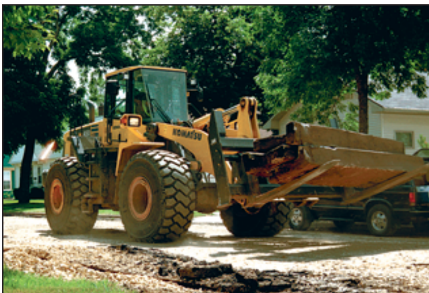
The operator of a Komatsu WA450-5 uses forks to move demolition debris at Three Rivers Construction's underground utility project in River Falls, Wisconsin.
