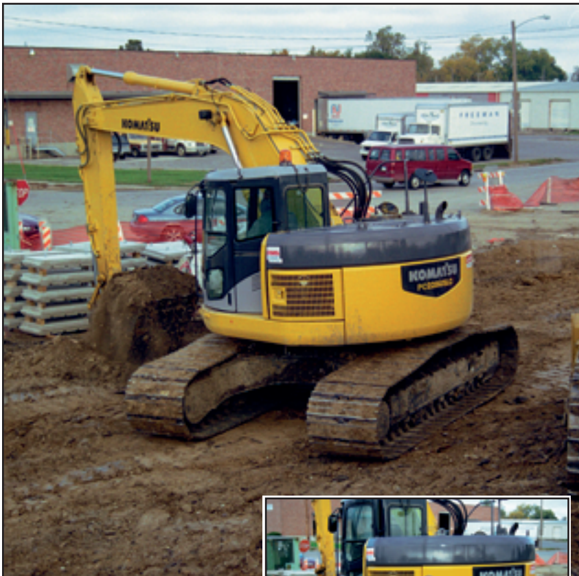
United Contractors Operator Jeremy Gilleland gets a full bucket with a Komatsu PC228 excavator during the company's work on the I-235 freeway project in Des Moines. He is pictured at right next to the unique excavator, which has a short tail swing radius, making the machine ideal for work in tight spaces.
