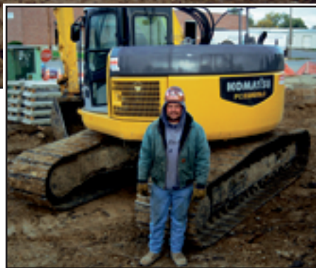
United Contractors Operator Jeremy Gilleland gets a full bucket with a Komatsu PC228 excavator during the company's work on the I-235 freeway project in Des Moines. He is pictured at right next to the unique excavator, which has a short tail swing radius, making the machine ideal for work in tight spaces.
