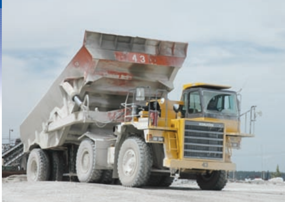
Drummond Dolomite uses six Komatsu HD325-6 haul trucks to carry materials from its pit to the crusher. The trucks were modified to carry as much as 75 tons over the six-mile haul. "We're able to haul more material at one time so our production cost isn't as high," said Plant Manager Gib Aikey.
