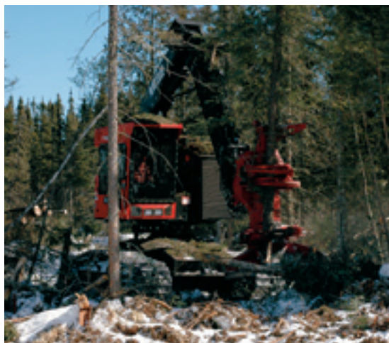
An operator for Knable Timber uses a Timbco 425EXL feller buncher from Komatsu Forest to fell trees.
