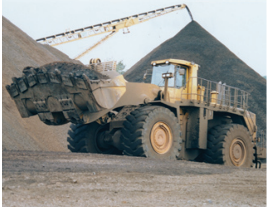
RMS offers the full line of Komatsu machines, from compact utility equipment to giant mining models. RMS customer Ulland Brothers uses its Komatsu WA800-3 wheel loader equipped with a 14.4-cubic-yard bucket to charge its crushing plant.
