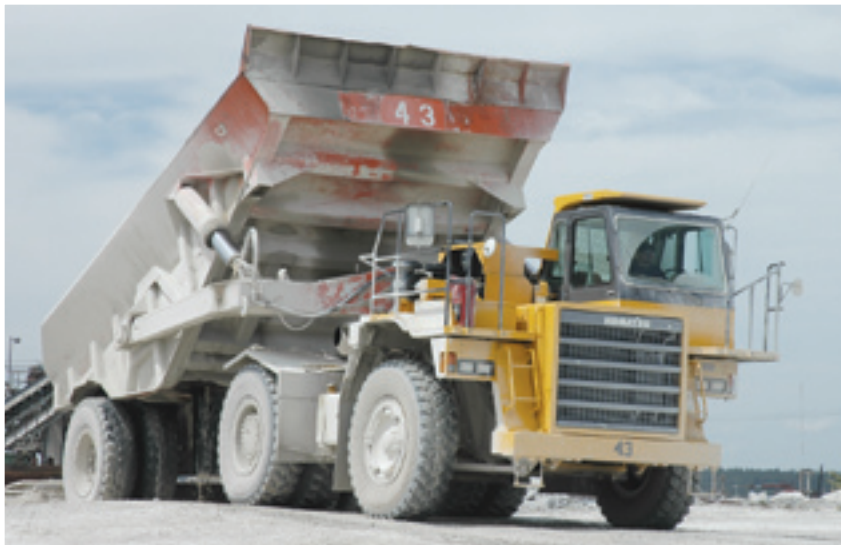
Drummond Dolomite turns to RMS for much of its heavy equipment needs, including this Komatsu HD325 haul truck. The company has six HD325s, which were modified to carry as much as 75 tons.
