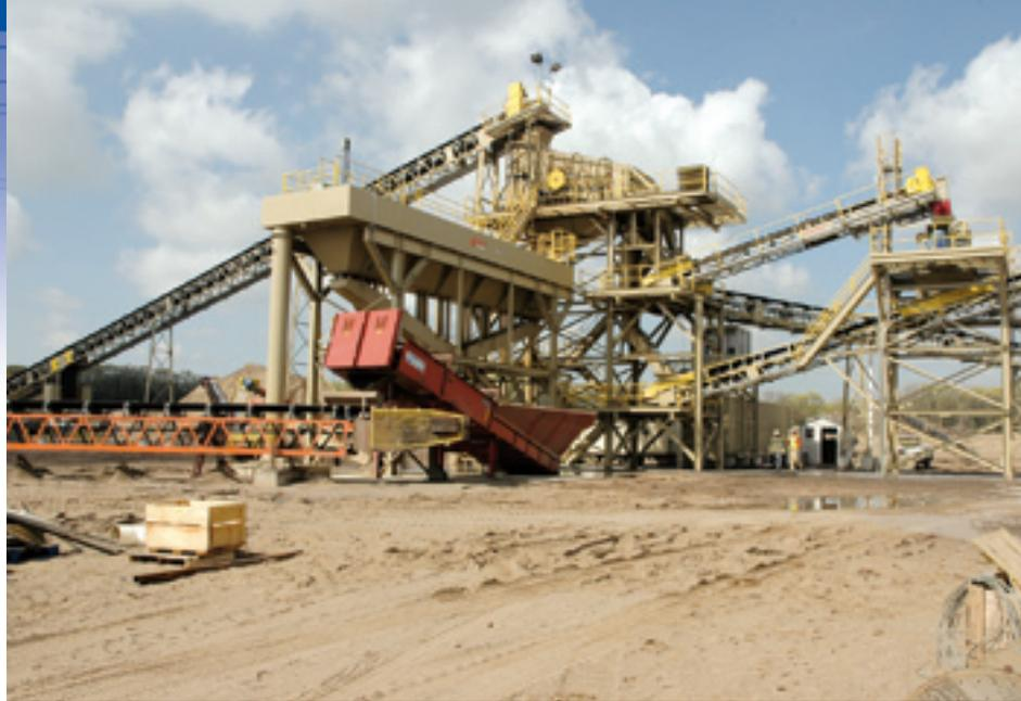
New Kolberg-Pioneer equipment at Aggregate Industries’ 600-acre Elk River Plant includes an 8’x20’, two-deck, dry, vibrating screen; two 8’x20’, three-deck, wet, vibrating screens; a 12’x48’ stationary classifying tank; a Pioneer 2500 vertical-shaft impactor; a 36-inch dewatering sand screw; and several pieces of stacking and conveying equipment.
