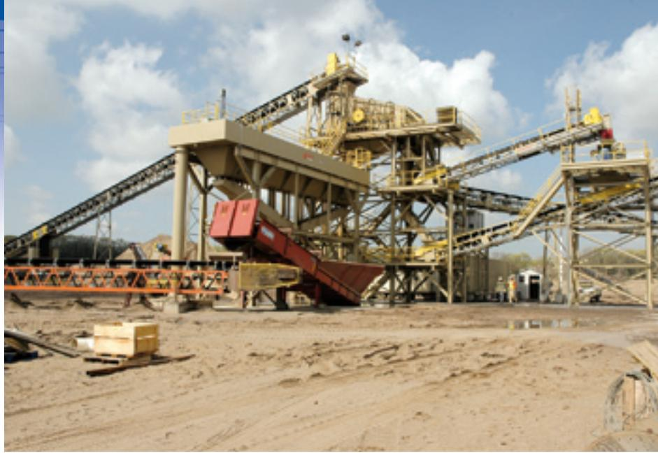
New Kolberg-Pioneer equipment at Aggregate Industries’ 600-acre Elk River Plant includes an 8’x20’, two-deck, dry, vibrating screen; two 8’x20’, three-deck, wet, vibrating screens; a 12’x48’ stationary classifying tank; a Pioneer 2500 vertical-shaft impactor; a 36-inch dewatering sand screw; and several pieces of stacking and conveying equipment.
