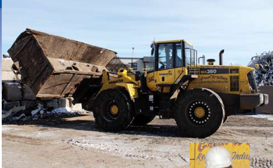
Operator Norman Bley moves a storage container with a Komatsu WA380-6 wheel loader. "That machine gives us a great deal of versatility because we can push piles and load with the bucket one minute and the next pick up bales or storage containers with the forks," said COO Jeff Kempin.
