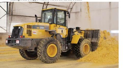
significant. That faster cycle time means we can get product out faster. That's partially because it has a very tight turn radius, so the operator can dig into the pile and get the bucketload to the truck with minimal movement.
