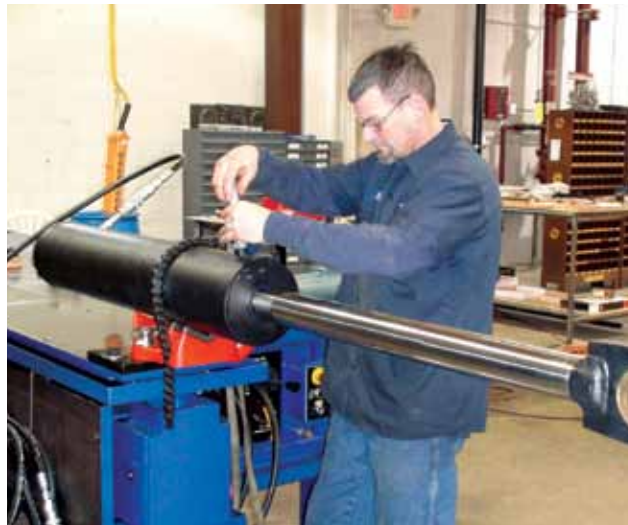
Sales and Operations Manager Rich Giese works on a cylinder using the tear-down bench, which allows RMS hydraulic shop personnel to take apart, repair and test cylinders from machines as large as a Komatsu PC1250LC excavator.
