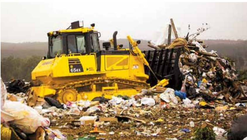
Komatsu's D65-17 waste-handler dozers are purpose-built with added guarding for working in tough conditions such as landfills. Blade options include SIGMA, power-angle-tilt and straight-tilt to match the user's need and maximize productivity.
