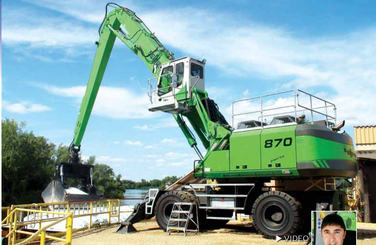
Operator Jerod Huppert unloads a barge with a SENNEBOGEN 870 M material handler. "It's ergonomically friendly," said Huppert of the 426-horsepower machine equipped with a 7-yard Rotobec clamshell bucket. "I like the joystick controls, and it's simple to use."
