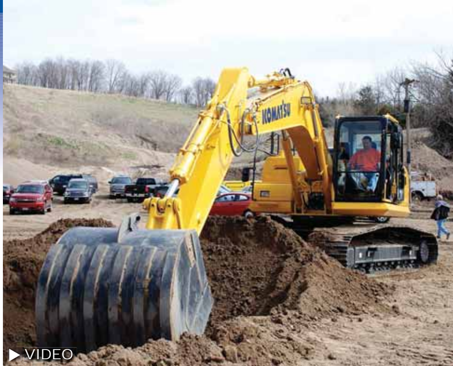
The PC210LCi-10 is the world's first intelligent Machine Control excavator, which semi-automatically limits overexcavation.
