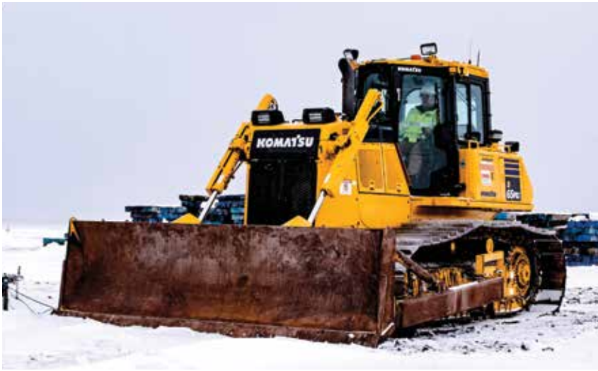
Using a Komatsu D65PXi dozer, a Northern Clearing operator packs frost and maintains a satellite equipment yard in Roseau, Minn.
