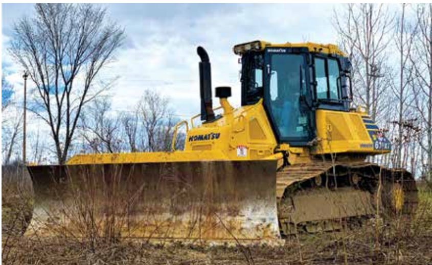
A George Bougalis and Sons, Co. crew member gets ready to use the company's Komatsu intelligent Machine Control D61PXi dozer on a road project in Chisholm, Minn. "The D61i eliminated our need to survey a site or use stakes, plus the operator doesn't need as much experience to be effective," said President Jim Bougalis. "It makes us 20 to 30 percent faster on jobs."
