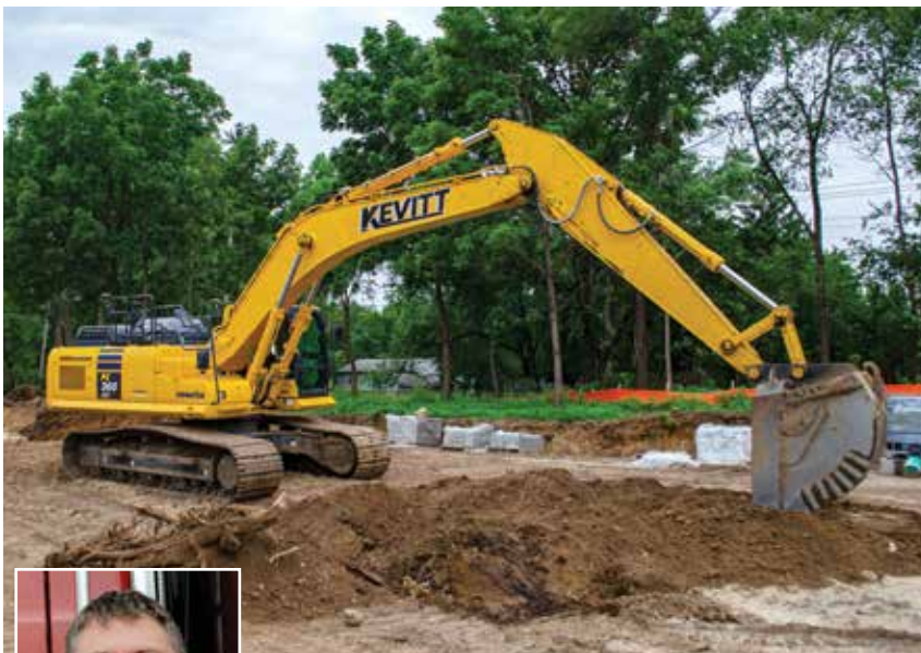
At a residential project in New Hope, Minn., a Kevitt Excavating operator uses a Komatsu intelligent Machine Control PC360LCi-11 excavator. "We save so much time with the intelligent excavators," commented Operations Manager Luke Masica. "Everything on the plans is uploaded to the machines."
