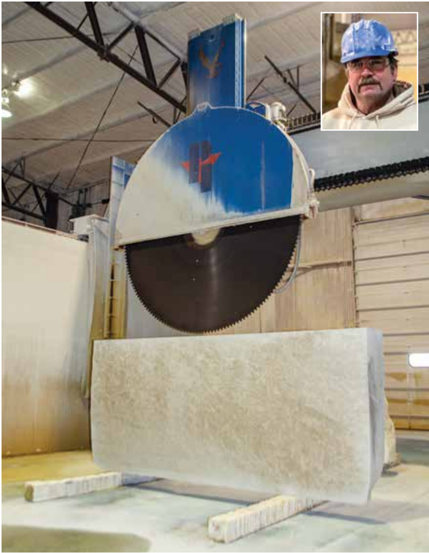
To cut large pieces of limestone, Weber Stone Company uses an 11.5-foot saw blade. "We can produce a slab of limestone in about 25 minutes," said Sawyer Dave Ammeter (inset).
