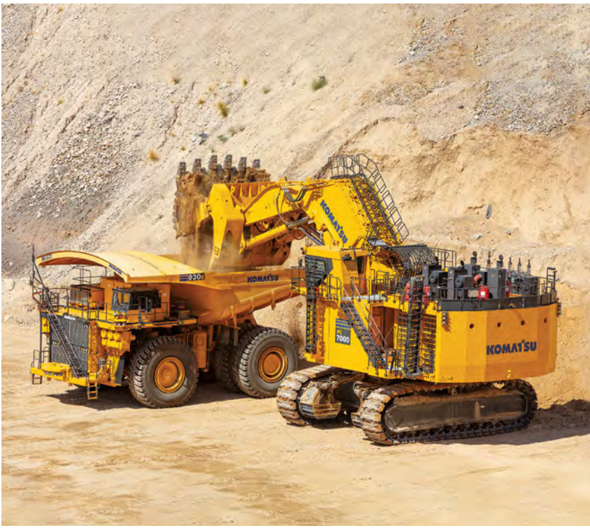
An Autonomous Haulage System (AHS) truck is loaded with a Komatsu hydraulic excavator at Komatsu's Arizona Proving Grounds. Customers using AHS recently surpassed 3 billion metric tons of material moved since the first AHS deployment in 2008.
