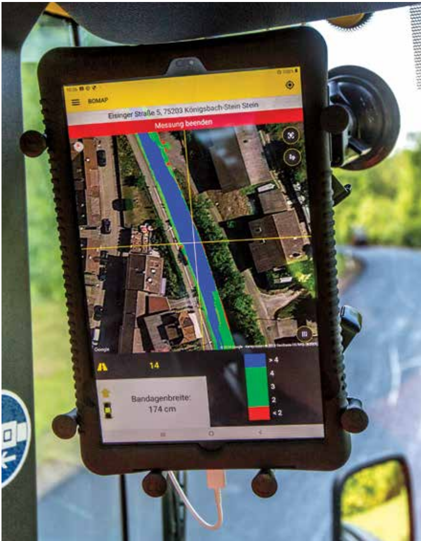
Smartphones and tablets with the BOMAP Connect app can be mounted inside the machine's cab, and operators can see real-time compaction data.
