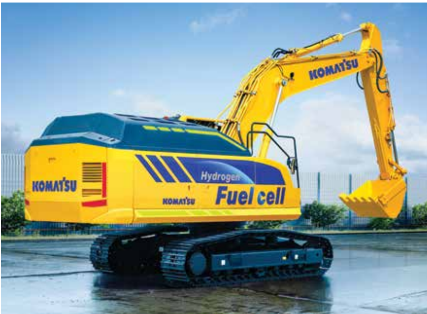
Komatsu has developed a concept machine for a medium-sized hydraulic excavator that combines a hydrogen fuel cell and other key Komatsu-developed components to help achieve carbon neutrality goals.
