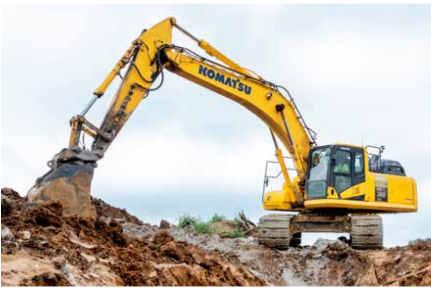
Komatsu IMC excavators go beyond simple guidance to semi-automatically limit over-excavation and trace a target surface.
