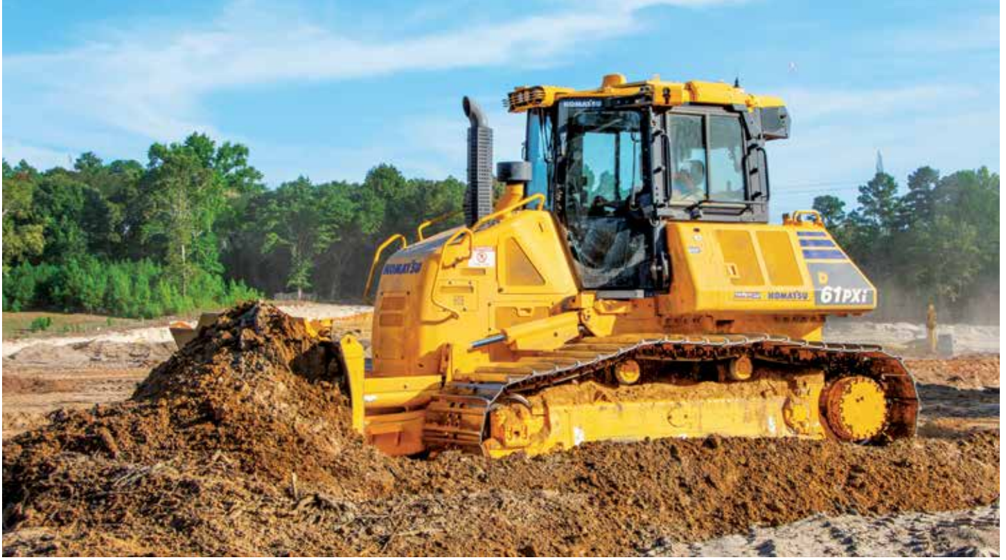
Komatsu's D61i-24 IMC 2.0 dozer is the second generation of the original IMC dozer introduced in 2013. Its features include proactive dozing control, lift layer control, tilt steering control, and quick surface creation.
