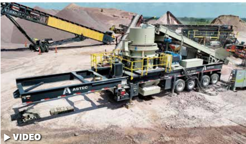
Last year, Duinick Inc. added an Astec KPI-JCI K500 cone crusher to its Scott Quarry aggregate pit in Hardwick, Minn. "We are producing about 200 tons more per hour," said Equipment Manager Courtland Acosta. "It's performing flawlessly."
