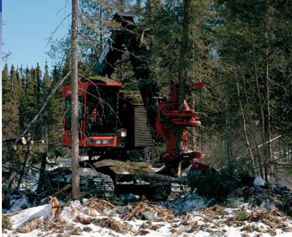
A Knaeble Timber operator uses a Timbco 425EXL feller buncher to fell trees on a project in Koochiching County. The machine features a cab-leveling system that allows easy operation on steep slopes and flat ground.
