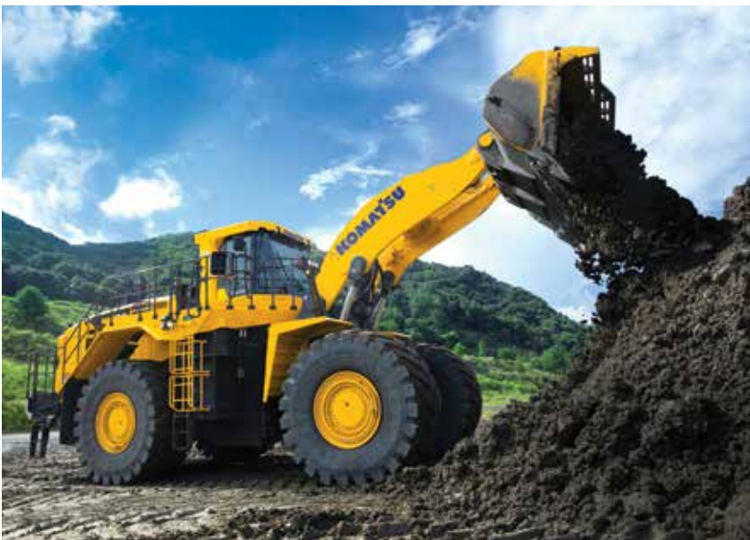
The WA700-8 is Komatsu's newest addition to its lineup of wheel loaders for quarry and aggregate operations.
