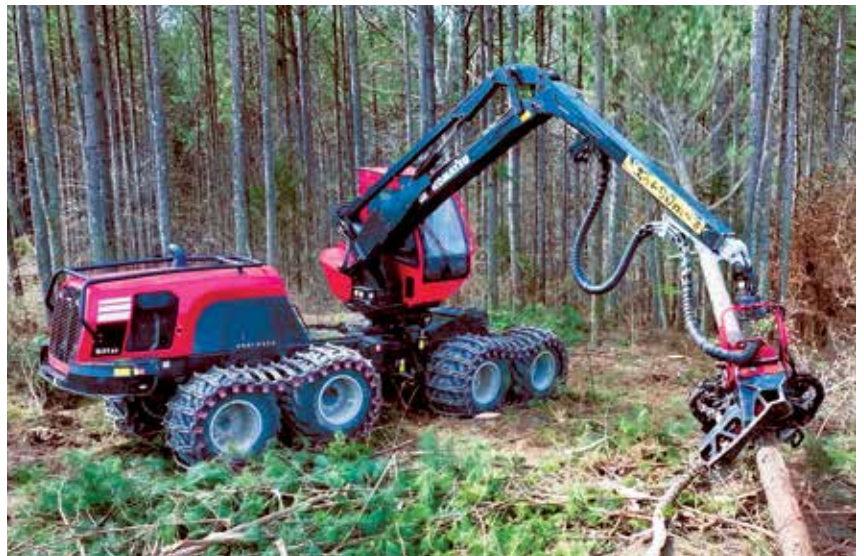
An operator uses a Komatsu 931XC harvester to cut timber to length for a logging operation.
